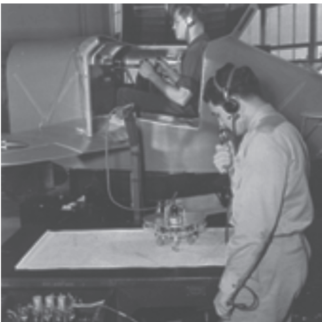
Figura 2. Simulador “Early Link Trainer” [4]
