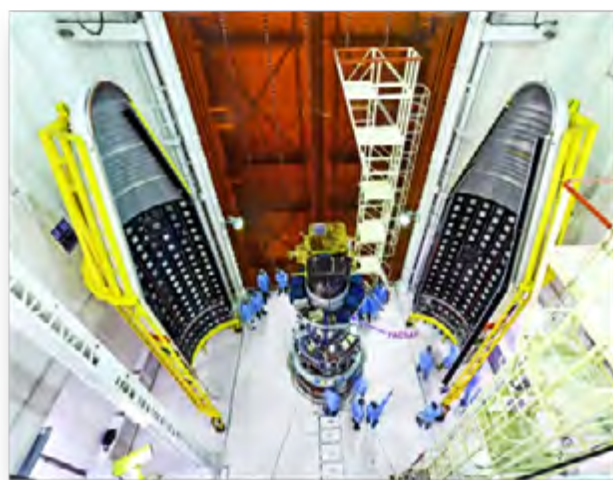
Figure 4. PSLV-C43 mission payload integration at Satish Dhawan Space Center.
